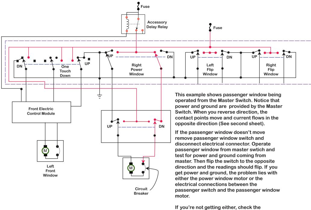
condition of the wires in the passenger door hinge area. If they're OK, then check for power and ground to the passenger window at the master switch.
